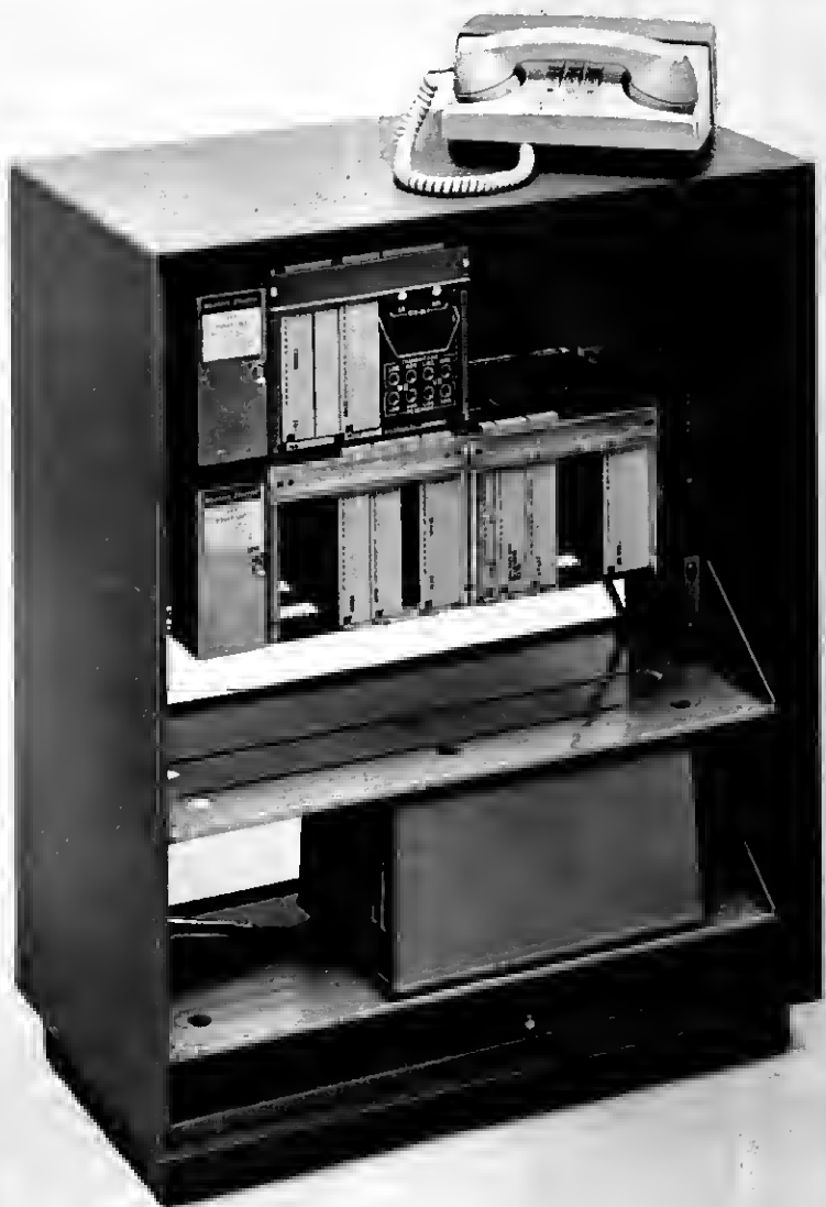
Fig. 5—Typical Data Station 303 used for 460.8-kb/s data transmission on the Picturephone network. Lower shelves provide space for the VLTU (shown in position), and optional equipment such as an automatic calling unit.
